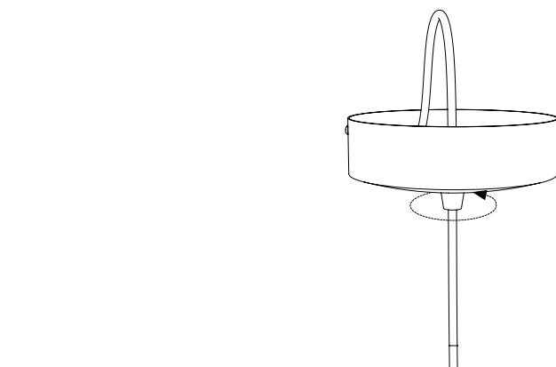
*Adjust the cable length and screw again the outer cord grip.
